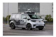
For the development of its autonomous ID. BUZZ AD<sup>1</sup>, Volkswagen Commercial Vehicles uses a new lidar sensor, Argo Lidar, which allows the vehicle to see objects from more than 400 meters away.
